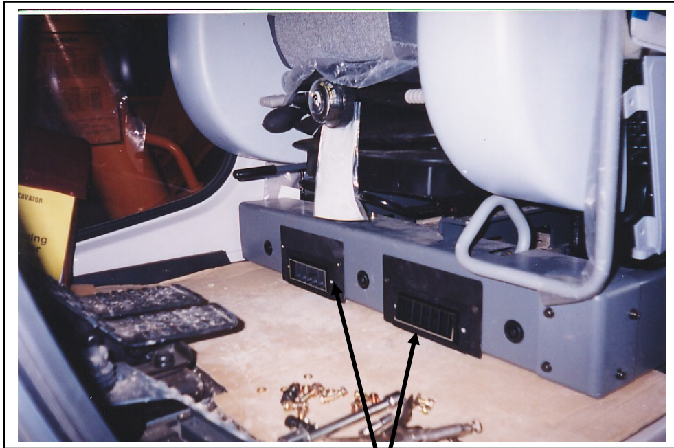
New louvers with hose adapters in place using existing hardware
